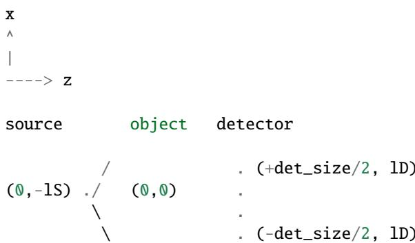
The algorithm computes all angular projections for discrete movements of the object. The position of the object is changed such that its lower boundary starts at  $(\text{det\_size}/2, 0)$  and its upper boundary ends at  $(-\text{det\_size}/2, 0)$  at increments of `shift_size`.
